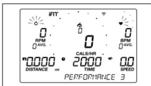
The maximum speed and the maximum resistance level for the workout will also appear in the display.
